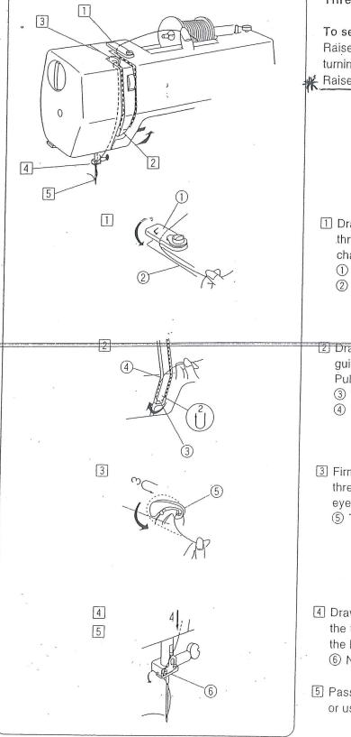
Threading the Machine - note direction of thread on specific
